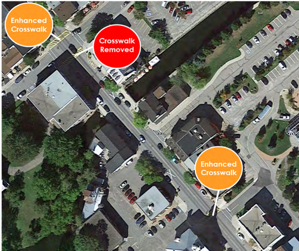
Figure 23 - Recommended Enhanced Crosswalk Locations
